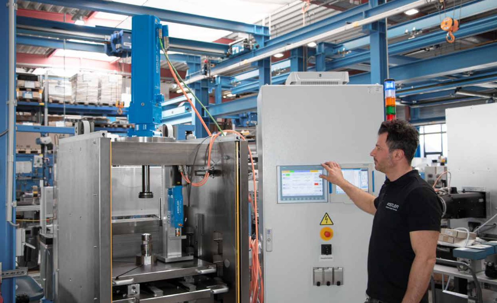
The Kistler test workstation comprising the frame, NC joining module, control cabinet with measurement technology, control and data acquisition unit
